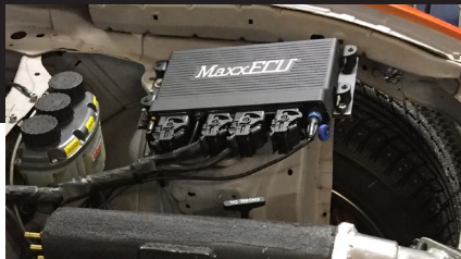
Example of a MaxxECU PRO installation.
